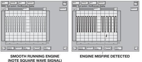
Depending on the level of misfire rate measured the ECM will illuminate the "Malfunction Indicator Light", deactivate the specific fuel injector to the particular cylinder and switch lambda operation to open-loop.
